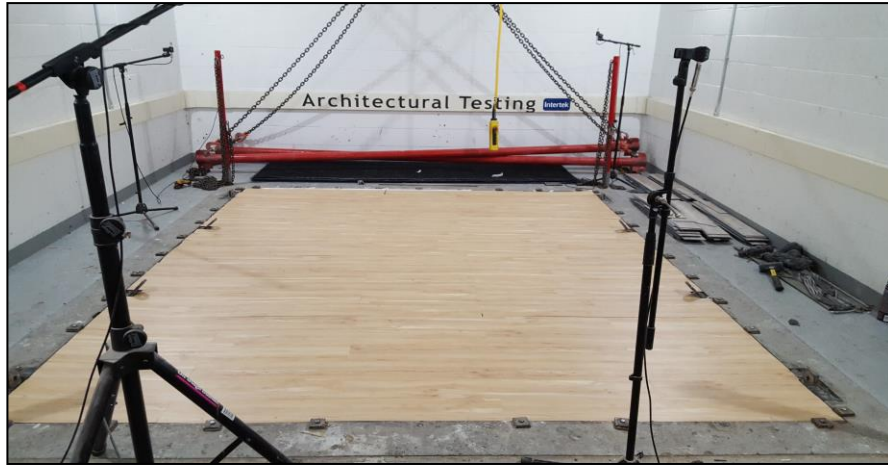
Source Room View of Test Specimen Installation
