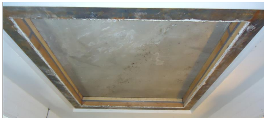
Receive Room View of Test Specimen Installation
